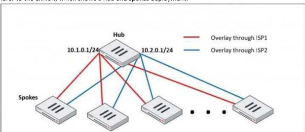
An administrator is deploying several spokes, including the BGP configuration for the spokes to connect to the hub.
