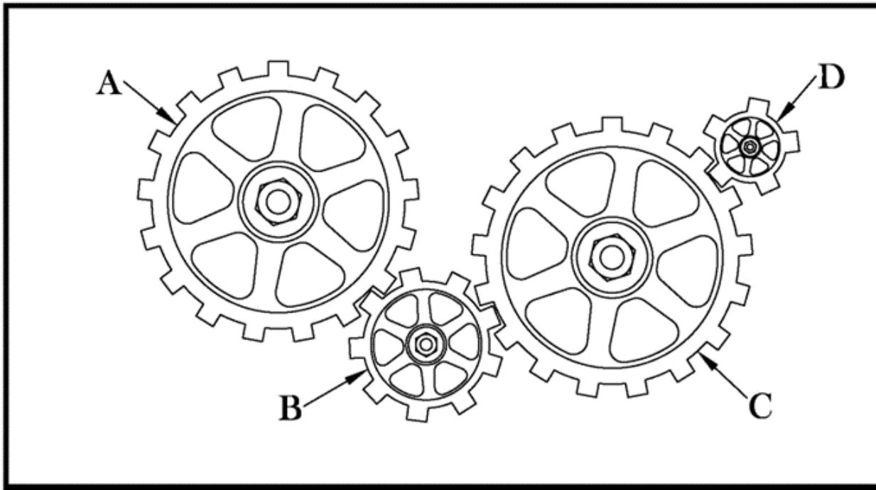
In the figure above, if gear C is turning at 100 RPM, which of the following is the best estimate for how fast gear B is turning?
