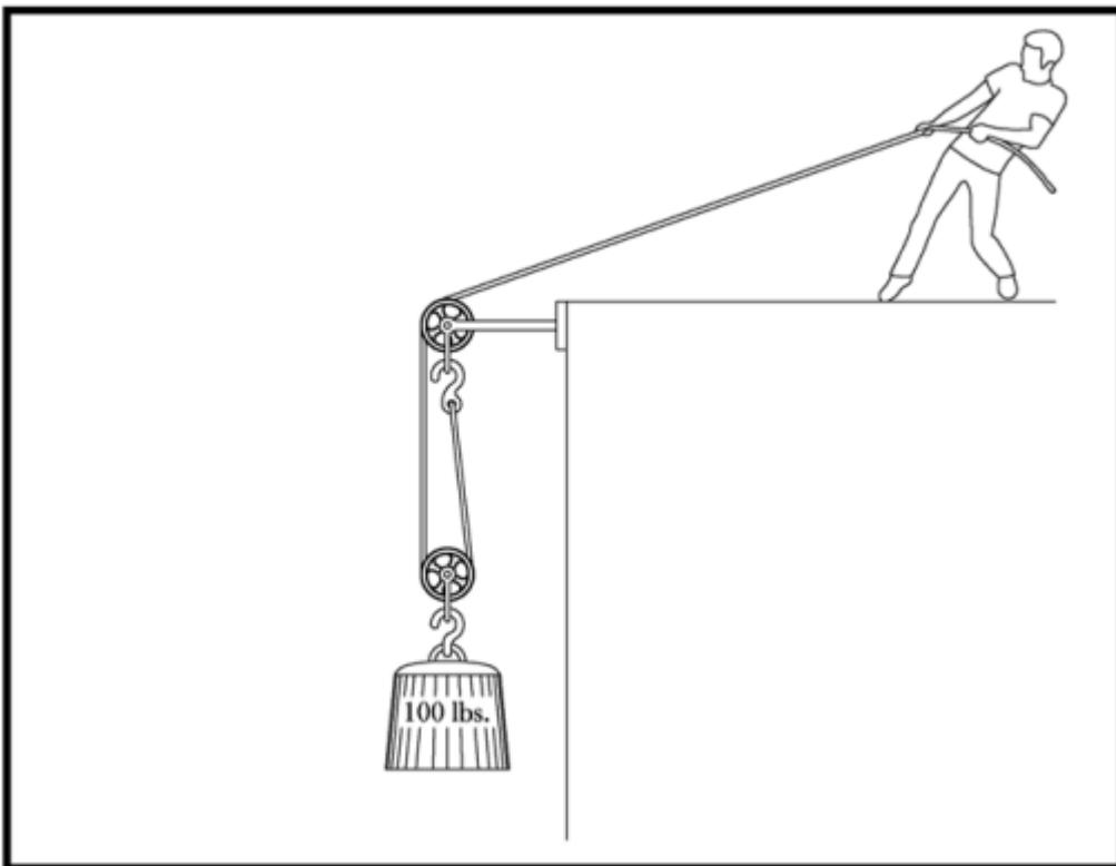
In the figure above, about how much force does the man have to pull with to raise the 100 lb weight?
