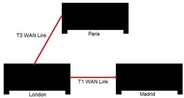
A company wants to implement replication using Dell EMC Data Domain systems in multiple locations. They want to replicate data at their London site to and from the Madrid site. In addition, the company wants to replicate data at the London site to and from the Paris site.
