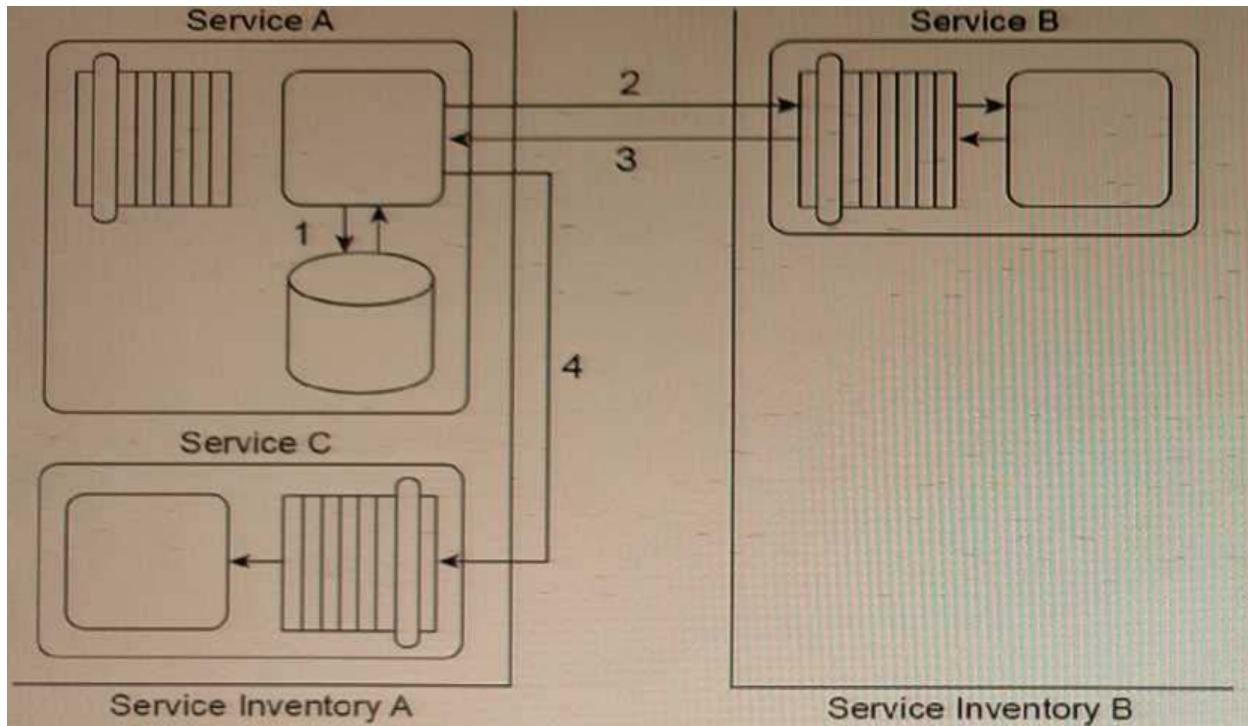
Service A is a task service that sends Service B a message (2) requesting that Service B return data back to Service A in a response message (3). Depending on the response received, Service A may be required to send a message to Service C (4) for which it requires no response.
