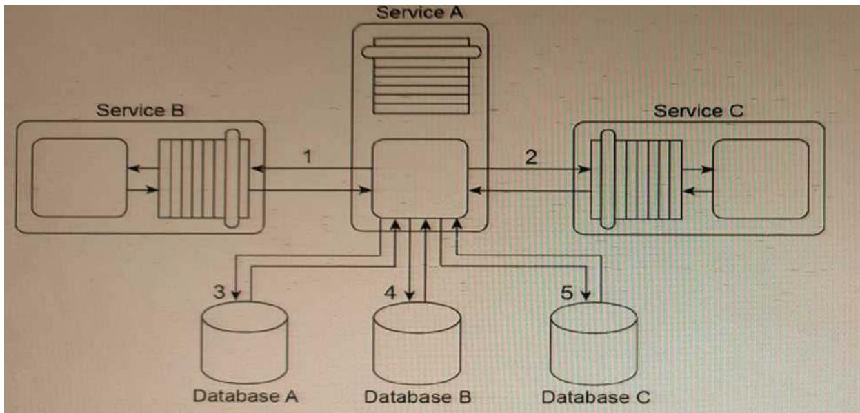
Service A is an entity service that provides a set of generic and reusable service capabilities. In order to carry out the functionality of any one of its service capabilities, Service A is required to compose Service B (1) and Service C (2), and Service A is required to access Database A (3), Database B (4), and Database C
