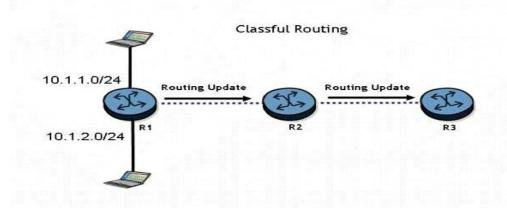
Routers R1 " R2, and R3 are running a classful routing protocol between them. Assuming that router R1 advertises all directly connected networks, how will these networks be represented in router R3's routing table?
