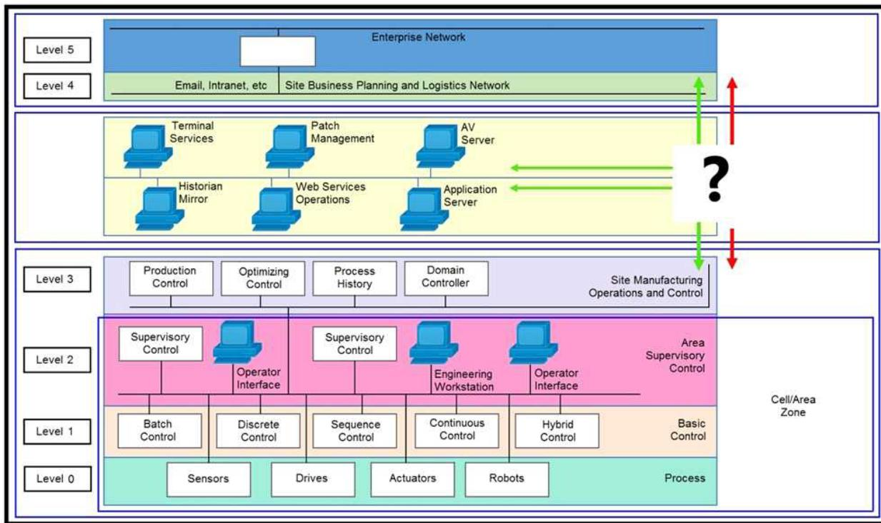
Which product must be positioned where the “?” is placed to connect these different network levels?
