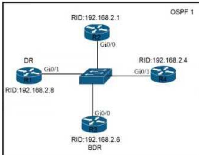
Refer to the exhibit. All routers in the network are configured. R2 must be the DR. After the engineer connected the devices, R1 was elected as the DR. Which command sequence must be configured on R2 to be elected as the DR in the network?
