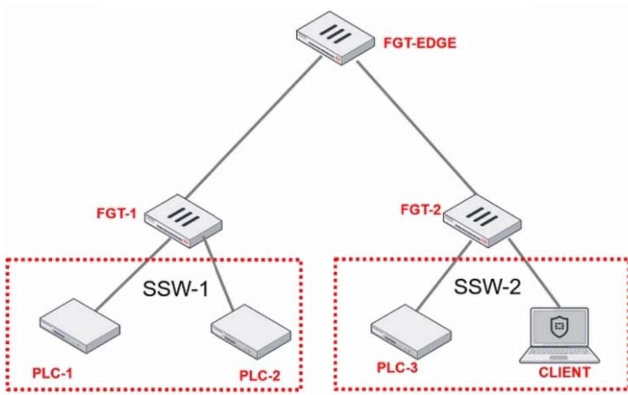
PLC-3 and CLIENT can send traffic to PLC-1 and PLC-2. FGT-2 has only one software switch (SSW-2) connecting both PLC-3 and CLIENT. PLC-3 and CLIENT can send traffic to each other at the layer 2 level. What must the operational technology (OT) admin do to prevent layer 2-level communication between PLC-3 and CLIENT? (Choose one answer)
