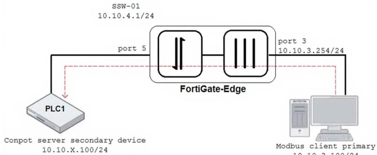
An OT architect has implemented a Modbus TCP with a simulation server Conpot to identify and control the Modbus traffic in the OT network. The FortiGate-Edge device is configured with a software switch interface ssw-01.
